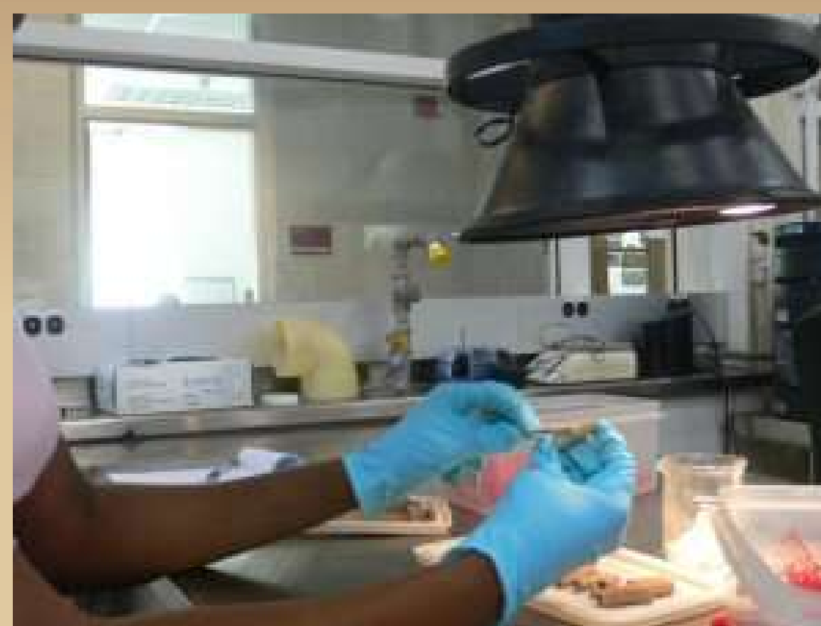
(Fig. 5, Cleaning pipe fragments using acetone)
